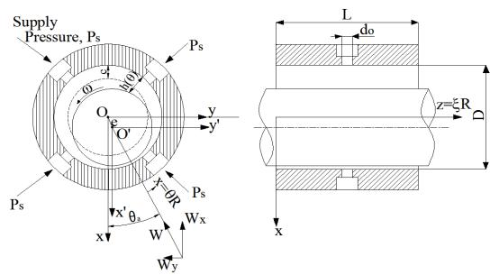
Figure 1. A hydrostatic journal bearing [28]
