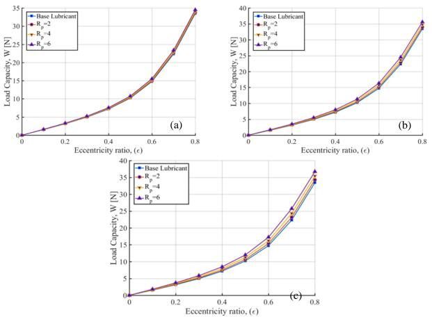
Fig. 3. Variations of the load capacity in regard to eccentricity ratio for different nanoparticle size, a)  $\varphi=0.25\%$ , b)  $\varphi=0.5\%$ , c)  $\varphi=0.75\%$
