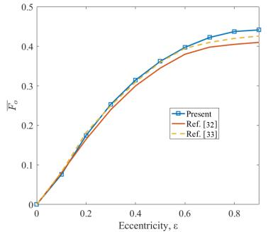
Figure 2. Variations of dimensionless fluid film forces with respect to eccentricity
