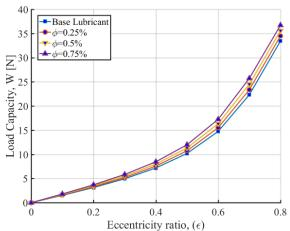
Fig. 4 Variations of the load capacity in regard to the eccentricity ratio for different volumetric ratios of the nanoparticle additive
