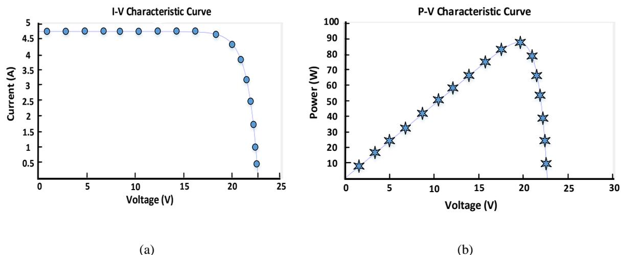
**Figure 2.** (a) P-V and (b) I-V Characteristics of the proposed solar PV Panel under loaded condition (1000 W/m<sup>2</sup>-25°C)
