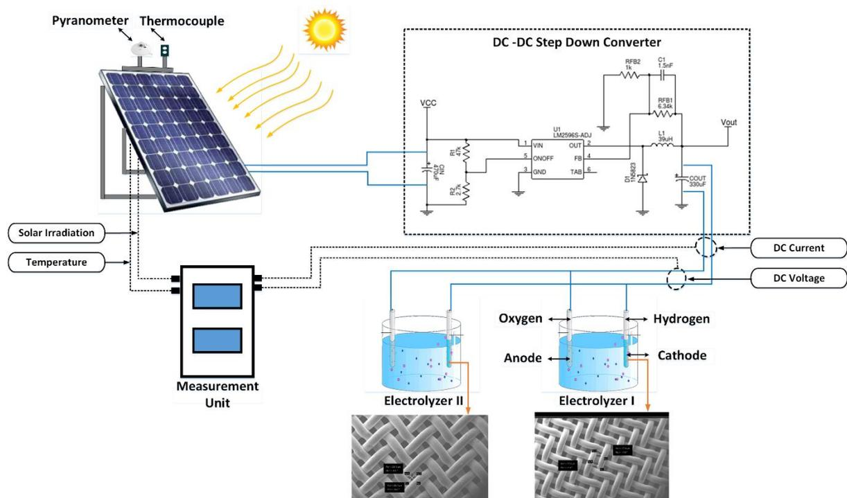
**Figure 1.** A solar PV combined-alkaline electrolysis hydrogen production system
