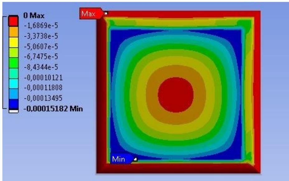
Fig. 6. Wear distribution on the surface of UC-20 Sample.
