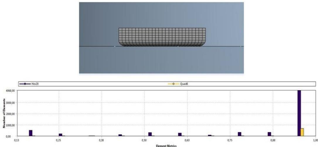
Fig. 2. Mesh view and mesh quality
