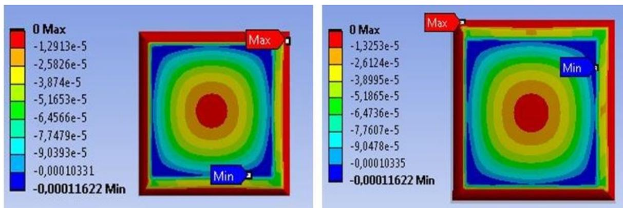
Fig.4. Wear distribution on the surface of UC-4&UC-8 Samples.
