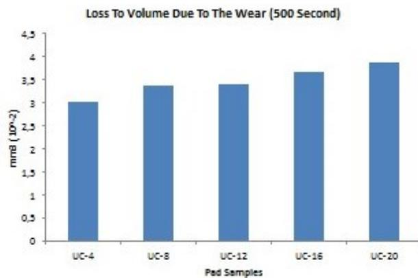
Fig. 3. Loss to volume due to wear of samples
