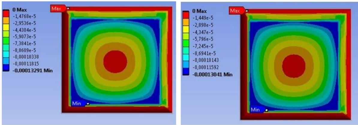
Fig. 5. Wear distribution on the surface of UC-12&UC-16 Samples.
