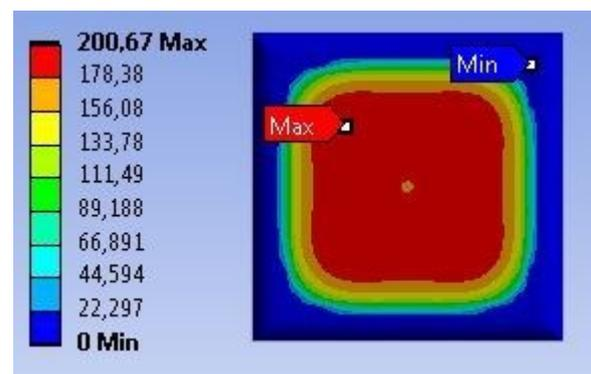
Fig. 10. Pressure distribution of the pad surface
