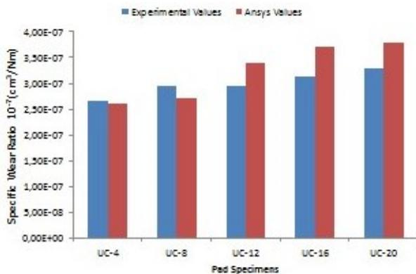
Fig. 8. Specific wear for experimental values and ANSYS values of specimens
