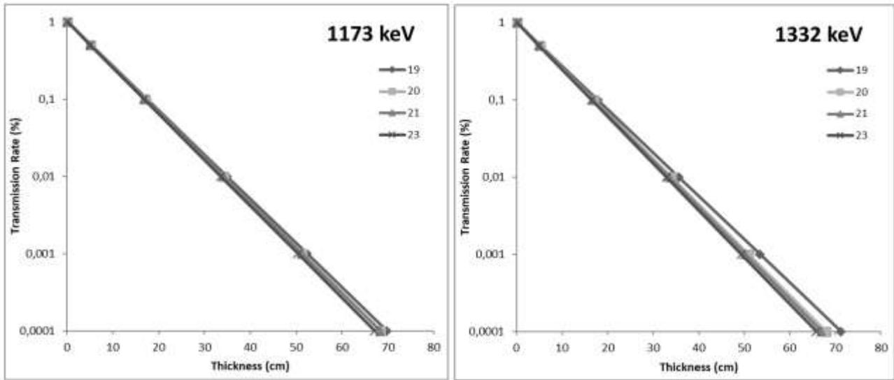
Figure 7. The transmission rate of the samples as a function of concrete thickness for 2<sup>nd</sup> group samples
