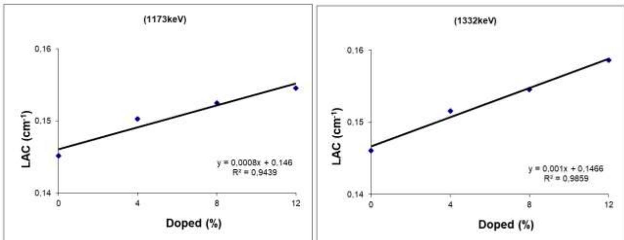
**Figure 3.** Variation of linear attenuation coefficient with energy for 1<sup>st</sup> group samples
