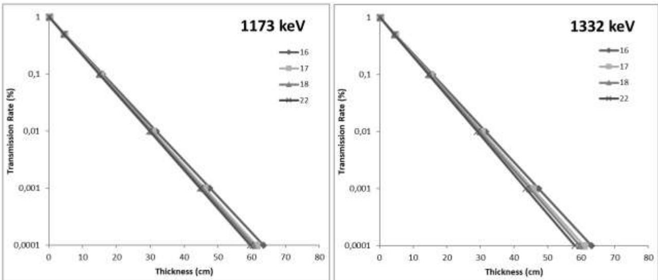
Figure 6. The transmission rate of the samples as a function of concrete thickness for 1<sup>st</sup> group samples
