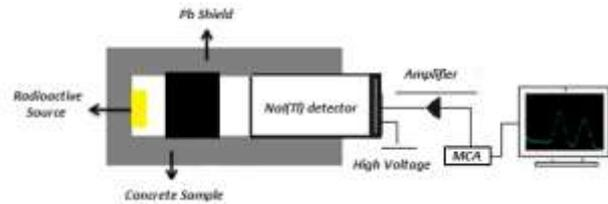
**Figure 2.** The schematic view of gamma-ray spectroscopy system
