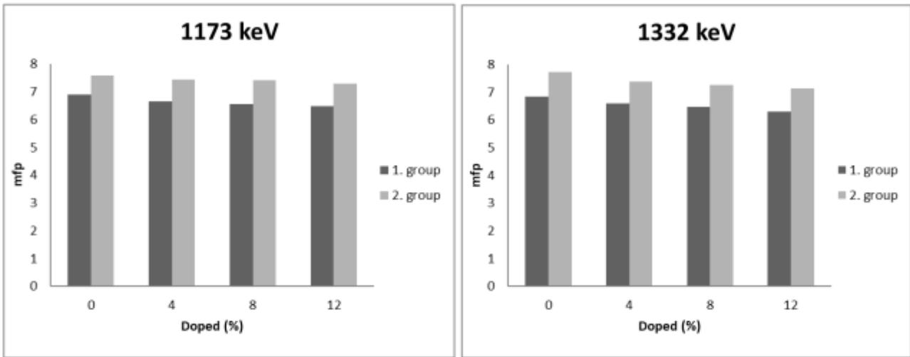
Figure 8. Mean free path- Marble powder ratio % changes measured for 1<sup>st</sup> and 2<sup>nd</sup> group samples
