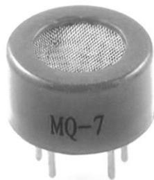
Figure 6. MQ7 air quality sensor
