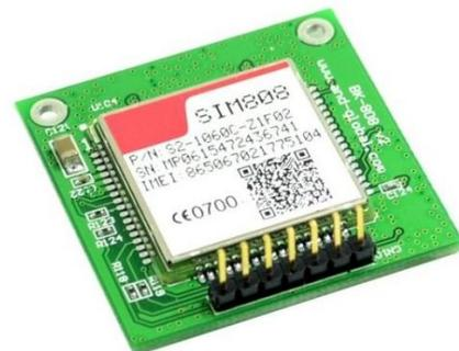
Figure 9. SIM808 GSM modem
