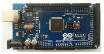
Figure 2. Arduino Mega 2560 Development Board.
