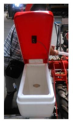
Figure 7. The montage of ultrasonic distance meter on seed tank
