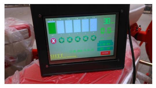
Figure 8. The boxed Nextion NX8048T070 TFT screen that used as graphical user interface
