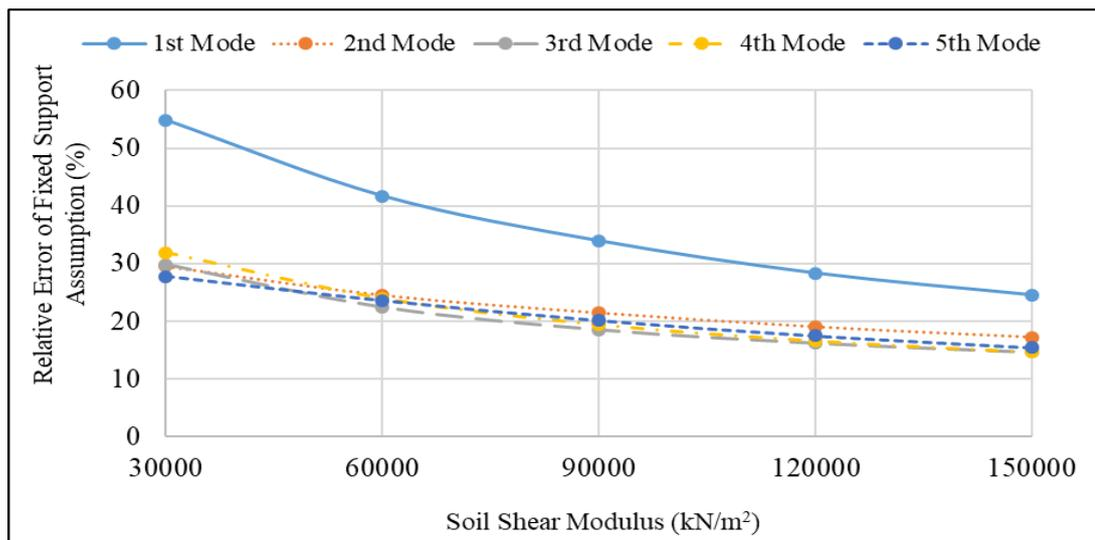
**Figure 2.** Relative error of fixed support assumption for different soil shear modulus values
