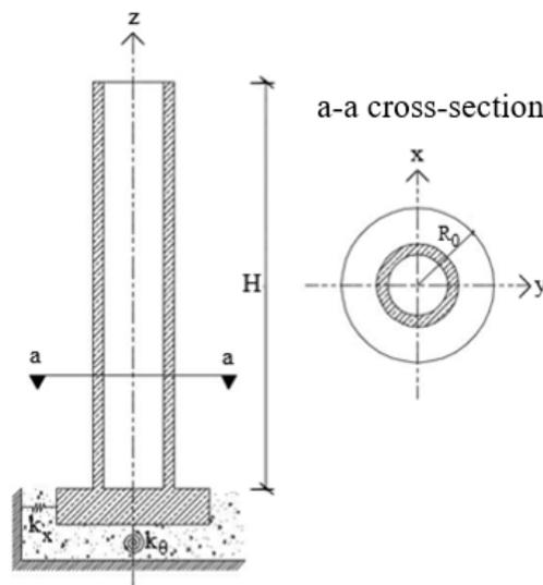
**Figure 1.** The chimney model with cross-section
