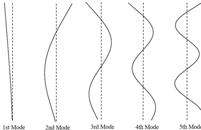
**Figure 3.** First five mode shapes of Timoshenko element chimney ( $G_s = 150000 \text{ kN/m}^2$ )
