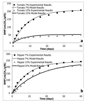
Figure 5. The simulation results to obtain  $k_R$  for anaerobic digestion of (a) tomato (b) pepper
