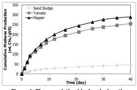
Figure 1. The cumulative biochemical methane production at SLR of 7%
