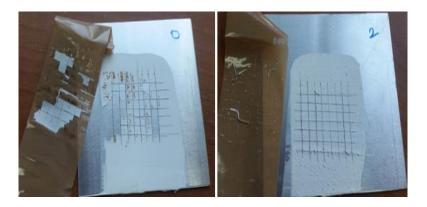
*Figure 21. Water based paint without aerogel as a paint additive*
