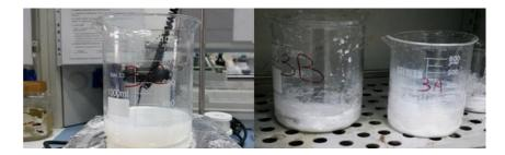
Figure 1. The gelation was occured after the polymerization step.
