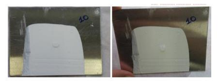
Figure 11. Sample with aerogel as a paint additive for water based paint
