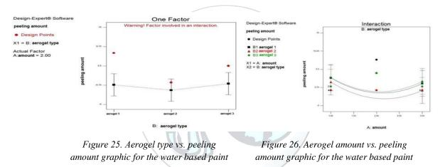
The graphics showed that the maximum adhesivity was obtained in case of using aerogel type 3 as a paint additive and the minimum adhesivity was obtained with the utilization of aerogel type 2. In addition to this, it has been observed that peeling amount decrease with the increasing amount of aerogel utilization.
