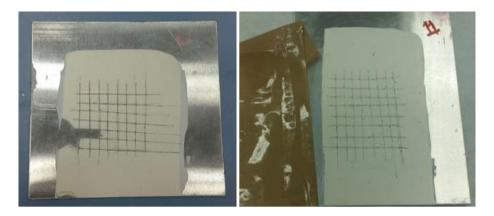
Figure 23. Solvent based paint without aerogel as a paint additive
