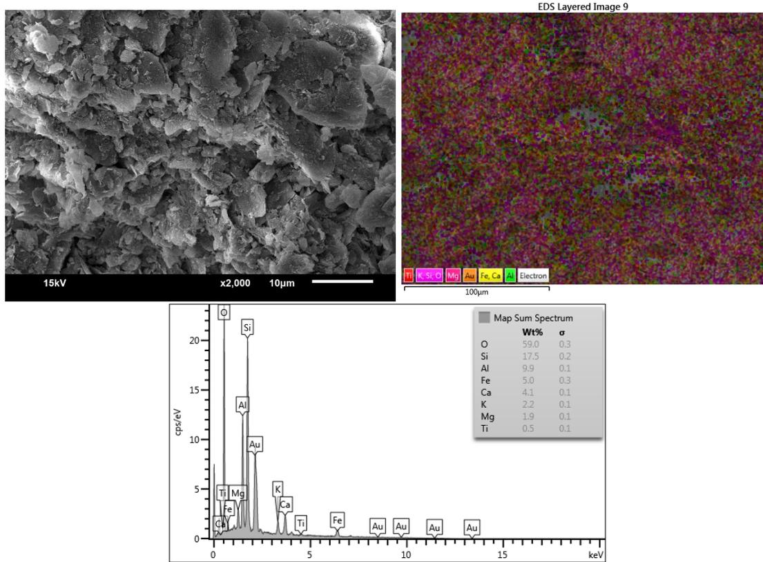
Fig. 8. SEM image, EDS spectrum, EDS mapping images for soil without lime
