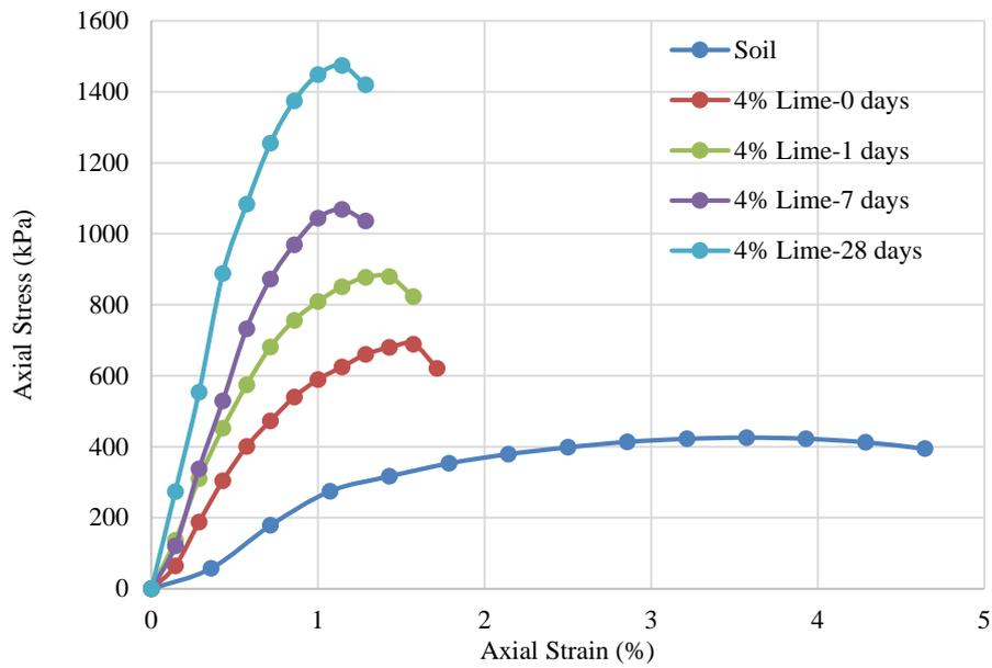
Fig. 6. Unconfined compressive strength change of soil prepared with %4 lime by weight for kept in desiccator.
