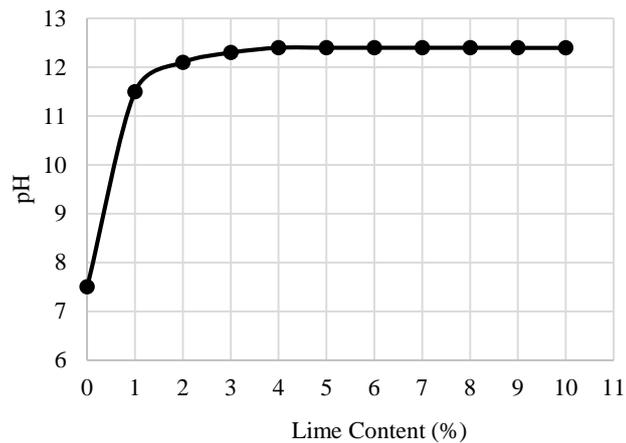
Fig. 2. pH values at various lime contents
