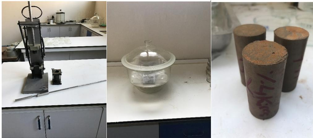
Fig. 1. Specimen preparation, desiccator curing and soaked specimen.
