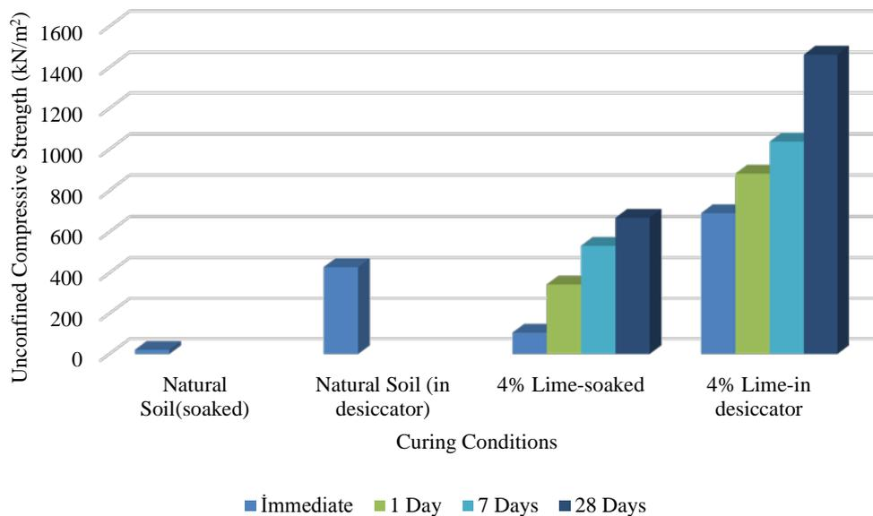
Fig. 5. Unconfined compressive strength change with curing time for different curing conditions.
