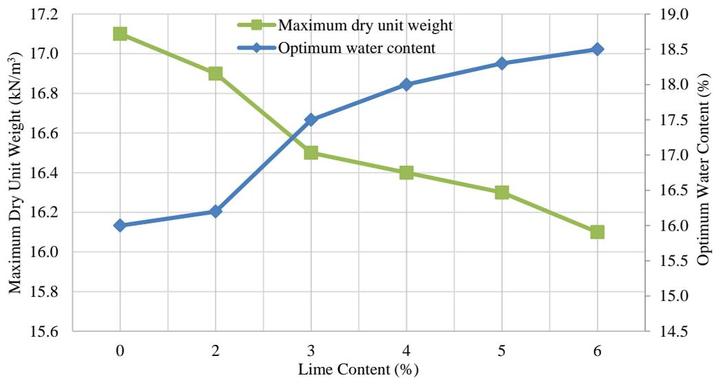
Fig. 3. Maximum dry unit weight and optimum water change for different lime percentages.
