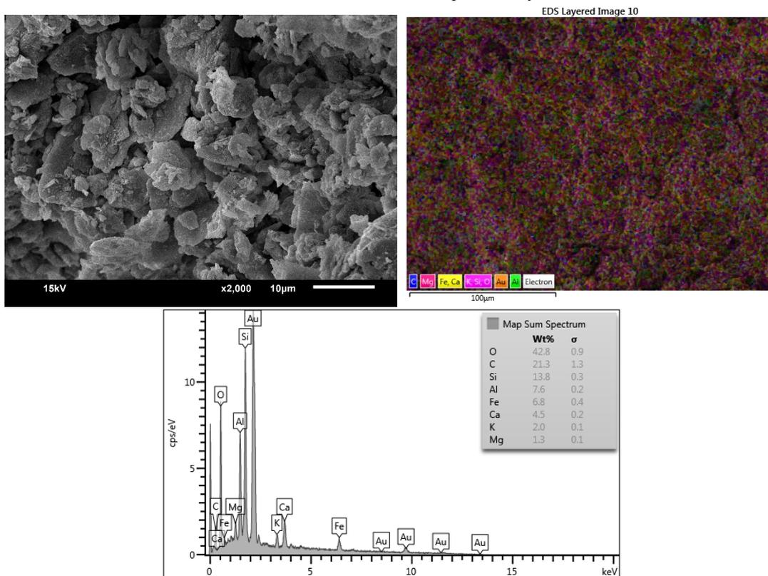
Fig. 9. SEM image, EDS spectrum, EDS mapping images for soil with 4% lime (for 28 days curing period)
