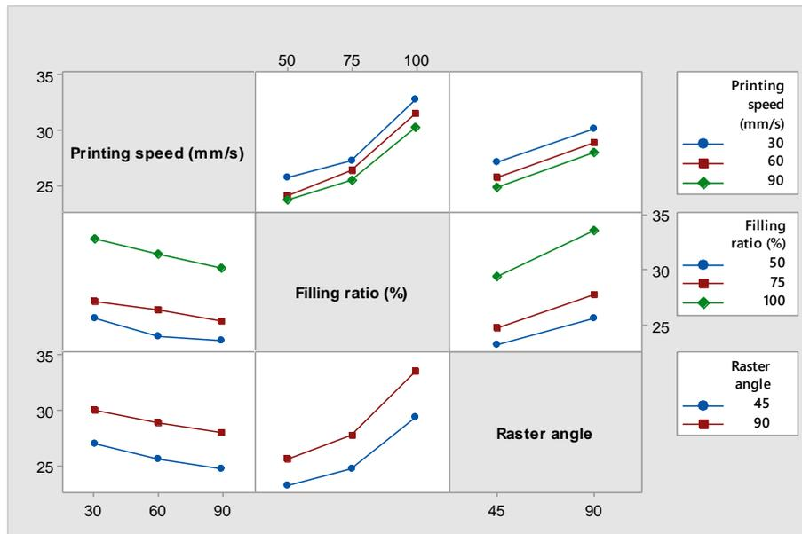
**Figure 2.** Tensile strength changes according to production parameters
