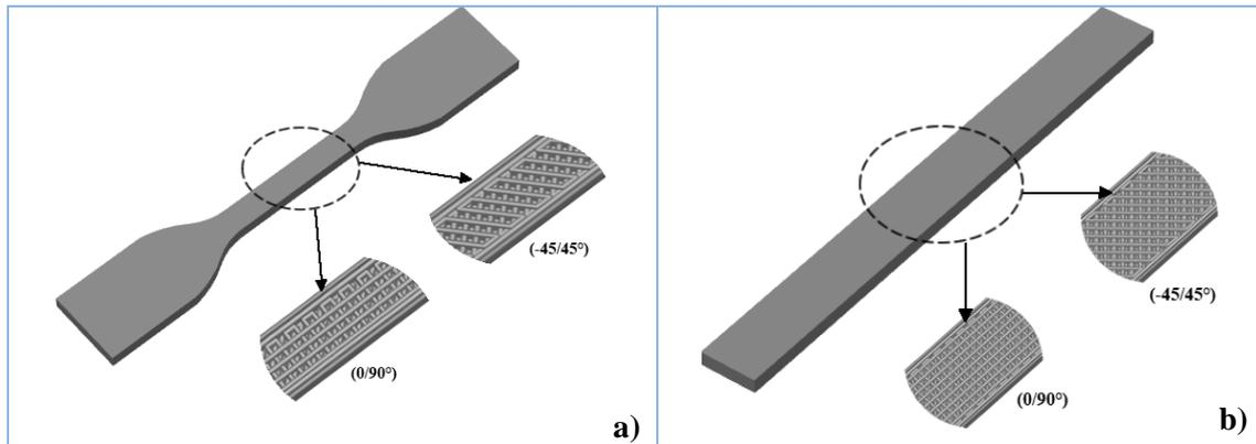
**Figure 1.** Sample 3D models; a) Tensile, b) Bending
