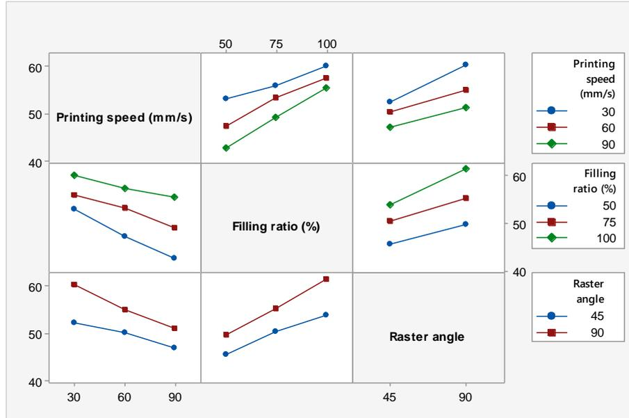
**Figure 3.** Bending strength changes according to production parameters.
